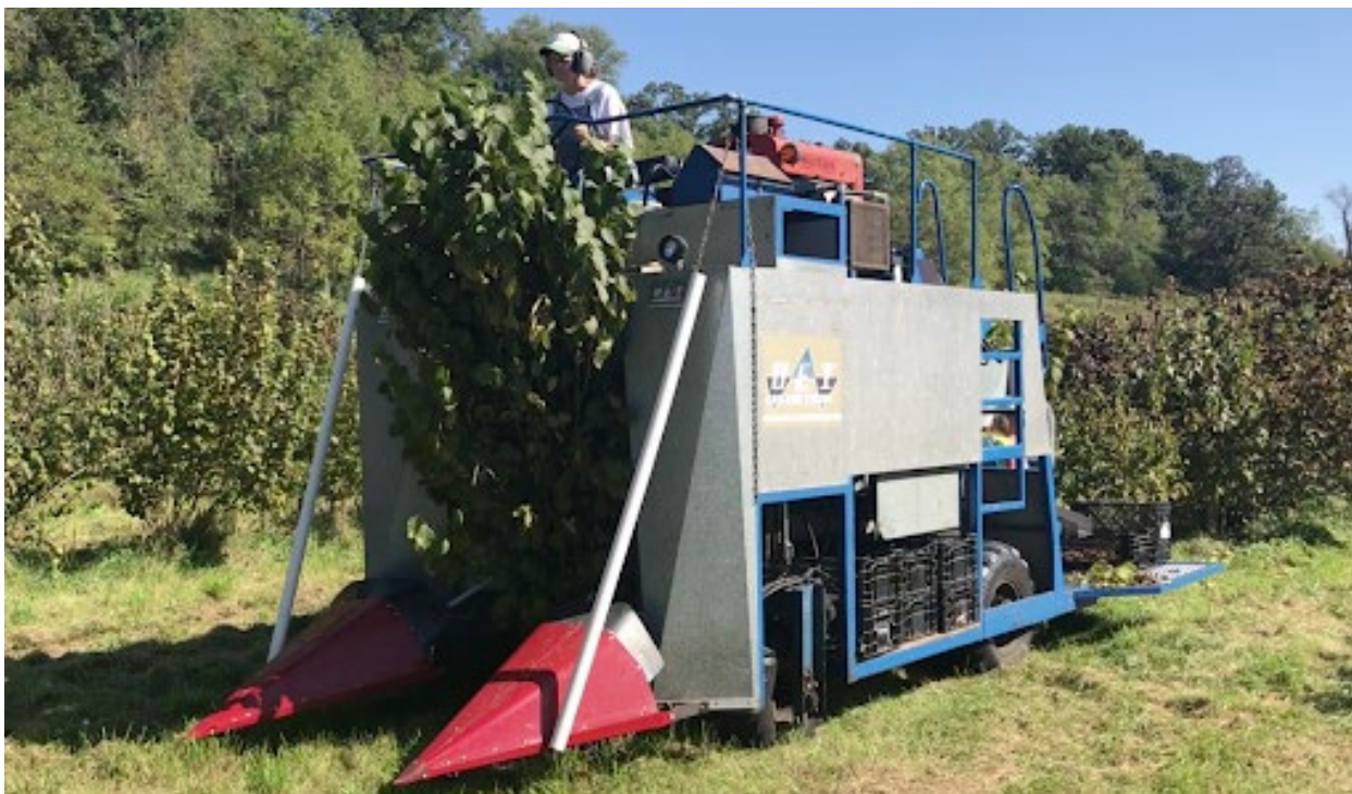
UMHDI has initiated a program to develop an optimized straddle-type harvesting system for hedgerow hazelnuts. In 2018, this slapper-type unit was trialed in multiple locations.
